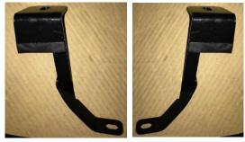
5. Remove the two bolts shown below with a 10mm Socket wrench for the bottom left and a 12mm Socket wrench for the bottom right. Once bolts are removed, carefully orient the bracket from the front of the vehicle, through the gap between the hood and the fender, and onto the two bolt locations. Take whatever precautions necessary (i.e. masking tape). Replace bolts and tighten. Use 10mm open-end wrench for bolt in bottom left picture. Repeat for opposite side of the vehicle.
