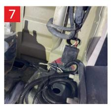
STEP ONE ROUTE THE CHMSL EXTENSION HARNESS THROUGH THE TOP HOLE IN THE CORNER PILLAR, BEHIND THE TAILLIGHT, AND THROUGH THE HOLE AT THE BOTTOM OF THE TAILLIGHT WELL. REFER TO PICTURE [1, 2, 3]
